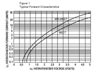
Instantaneous Forward Current - Amperesversus Instantaneous Forward Voltage - Volts
