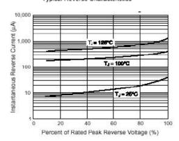
Figure 2 Typical Reverse Characteristics
