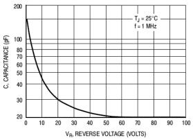
Figure 6. Typical Capacitance
