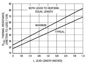
Figure 5. Steady-State Thermal Resistance
