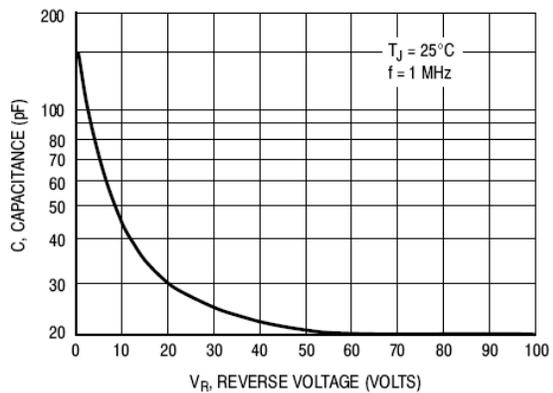
Figure 6. Typical Capacitance
