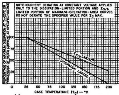
Fig. 1 - Derating curves for both types.
