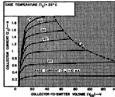
Fig. 5 — Typical output characteristics for both types.
