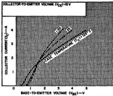
Fig. 4 — Typical transfer characteristics for both types.
