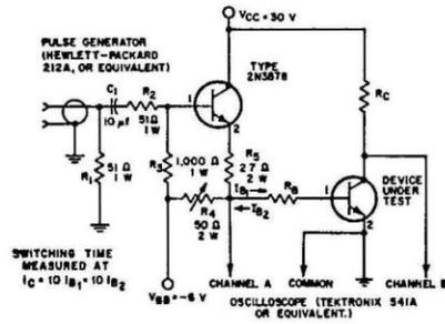
Fig. 9 — Circuit used to measure sustaining voltages, V<sub>CE0(sus)</sub> and V<sub>CE1(sus)</sub> for both types.
