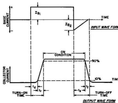
Fig. 12 — Phase relationship between input and output currents showing reference points for specification of switching times.
