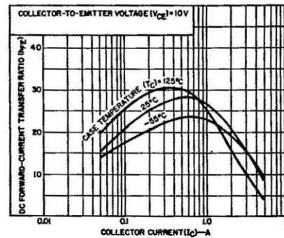
Fig. 2 - Typical dc beta characteristics for both types.
