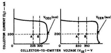
Fig. 10 — Oscilloscope display for V<sub>CE0(sus)</sub> and V<sub>CE1(sus)</sub> measurement.
