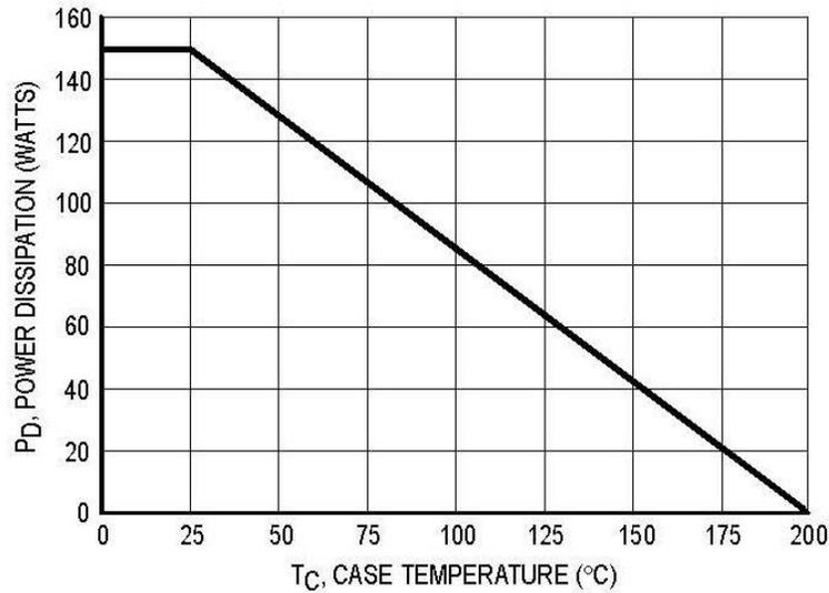
Figure 1. Power-Temperature Derating Curve
