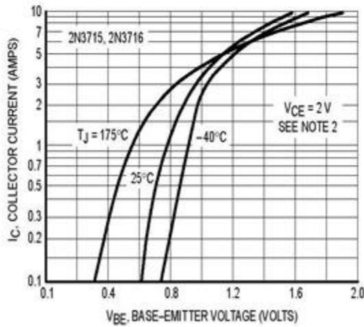
Figure 5. Collector Current-Voltage Variations
