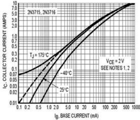
Figure 3. Collector Current versus Base Current
