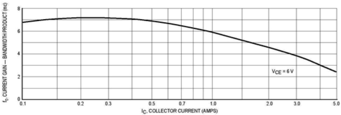
Figure 11. Current Gain — Bandwidth Product versus Collector Current
