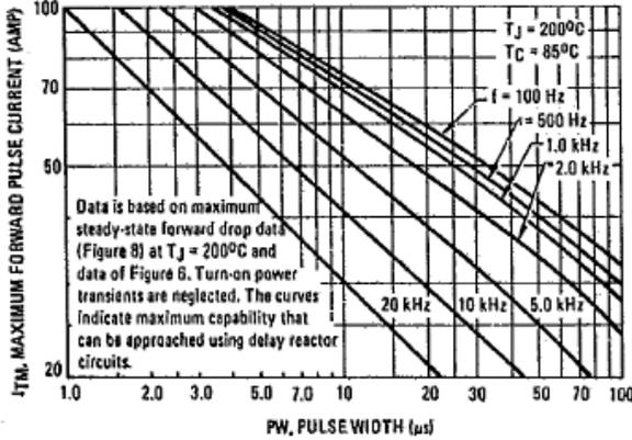
**DERATING USING TYPICAL SWITCHING LOSSES**
