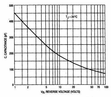
Figure 6. Typical Capacitance (Per Leg)
