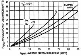
Figure 3. Forward Power Dissipation
