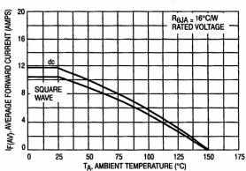
Figure 5. Current Derating, Ambient
