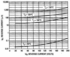
Figure 2. Typical Reverse Current (Per Leg)
