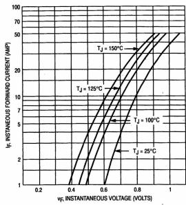
Figure 1. Typical Forward Voltage (Per Leg)
