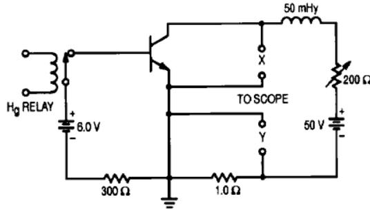
Figure 4. Sustaining Voltage Test Circuit
