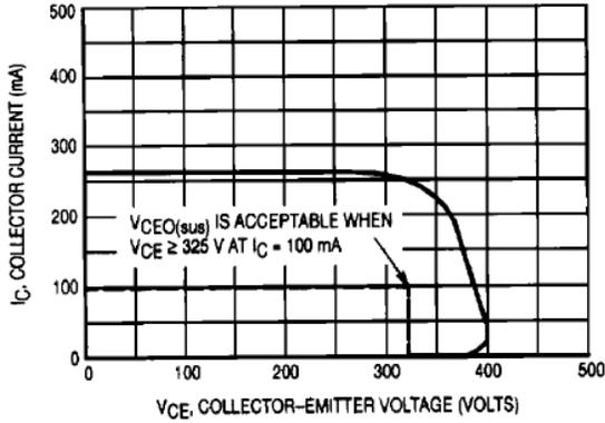
Figure 3. Sustaining Voltage Test Load Line
