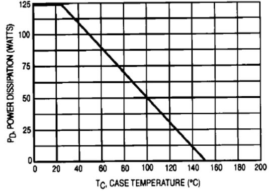
Figure 2. Power-Temperature Derating Curve
