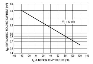
Figure 5. Typical Holding Current versus Temperature
